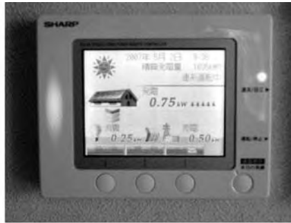
Energy consumption monitoring system
